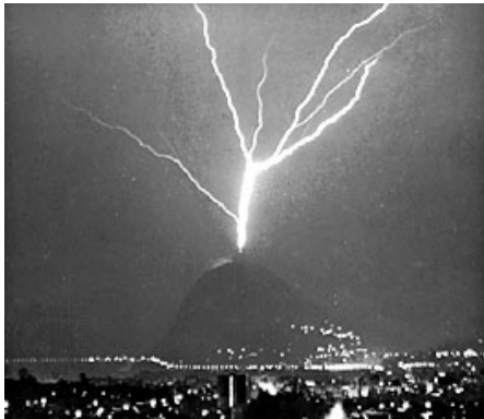
Fig. 4 - Picture of an upward lightning strike propagating from Berger’s TV tower on Mount San Salvatore.
